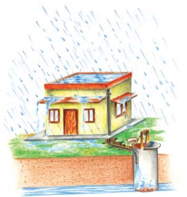
(b) Recharge through Abandoned Dugwell
